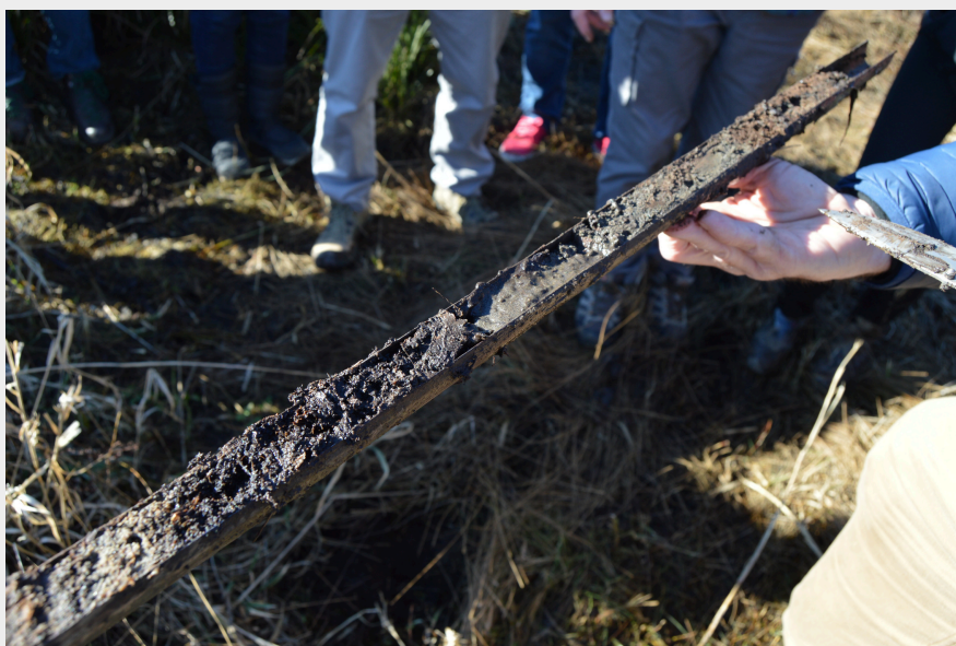
A sediment core showing the tsunami deposit layer
